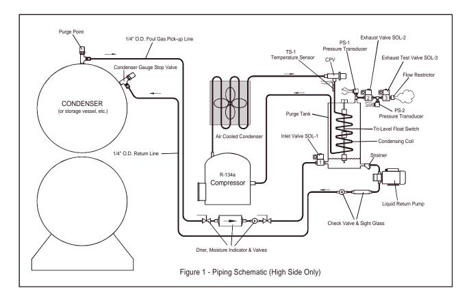
Figure 1 – Piping Schematic (High Side or Storage Vessel ONLY) Schematic for High---Low piping on the following page)
