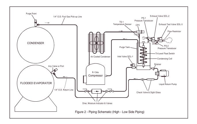
Figure 2 – Piping Schematic (High – Low Side Piping)
