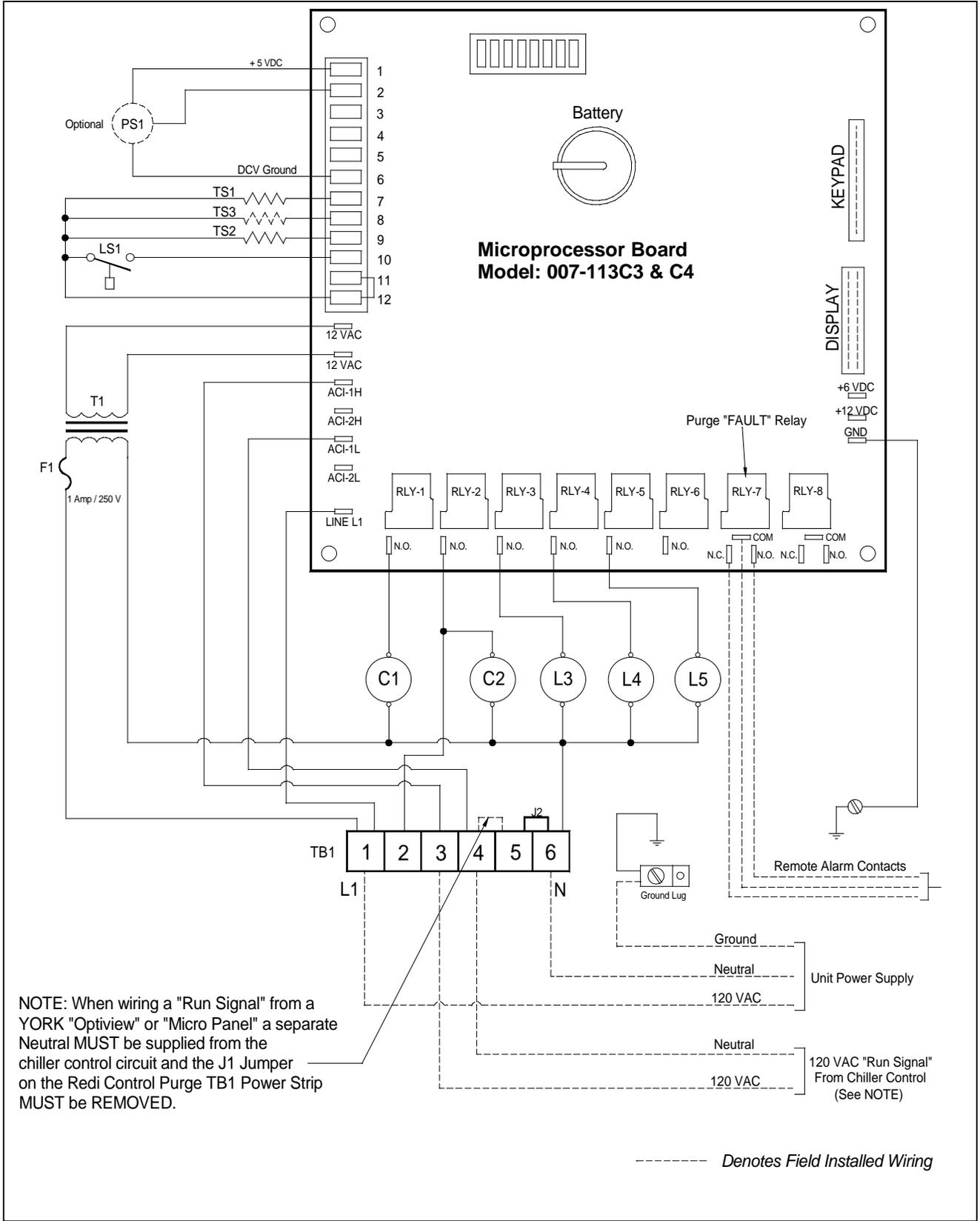
**(Figure 5A Wiring is for Purge replacement on a YORK Chiller)**
