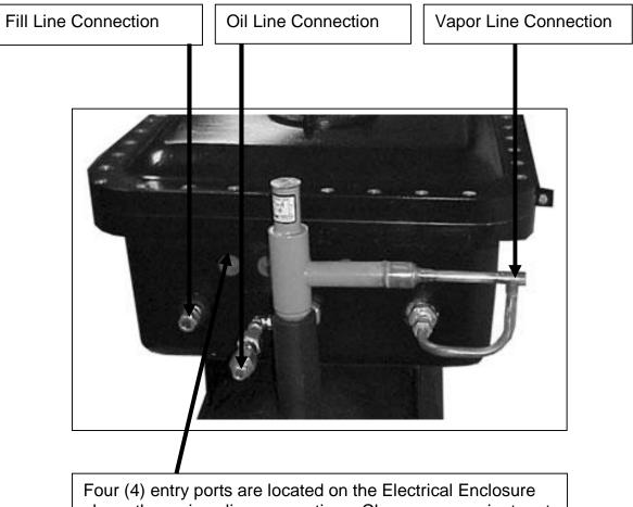
Four (4) entry ports are located on the Electrical Enclosure above the various line connections. Chose a convenient port for the Heater's electrical entry and a convenient port for the Power entry. Plug the remaining two ports.
