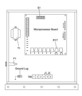
Figure 2 - Control Panel Interior
