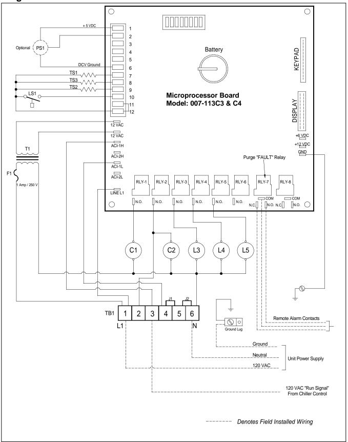
Figure 5A – Electrical ... (Figure 5A Wiring is for Purge replacement on a <u>YORK Chiller</u>)
