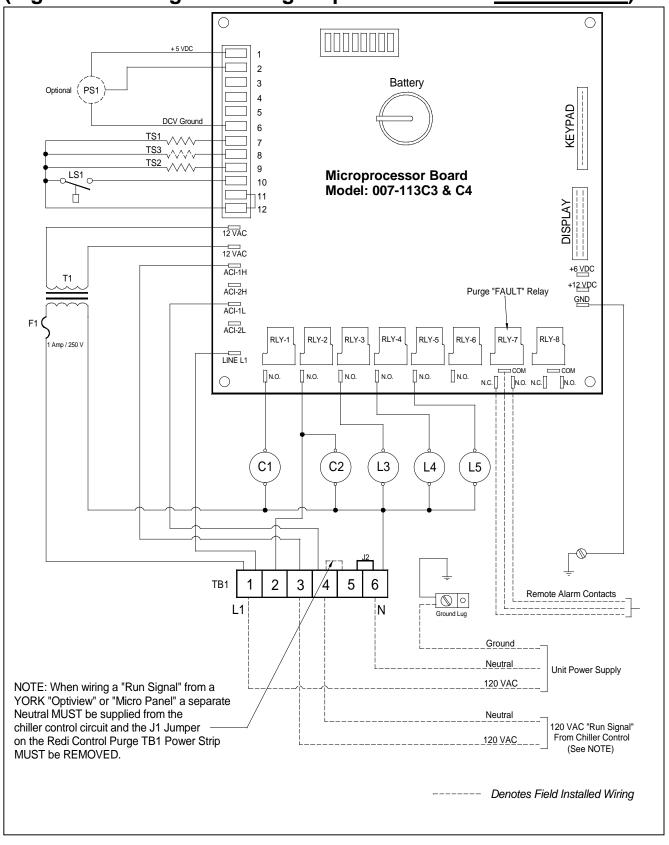
(Figure 5A Wiring is for Purge replacement on a YORK Chiller)
