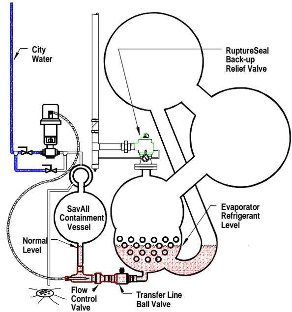
**Figure 1. - Chiller Idle, Pressure Normal**
