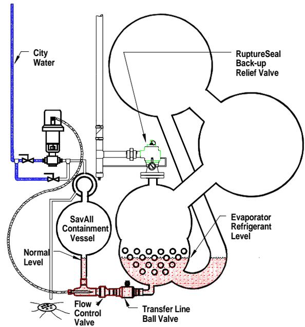
**Figure 1. - Chiller Idle, Pressure Normal**
