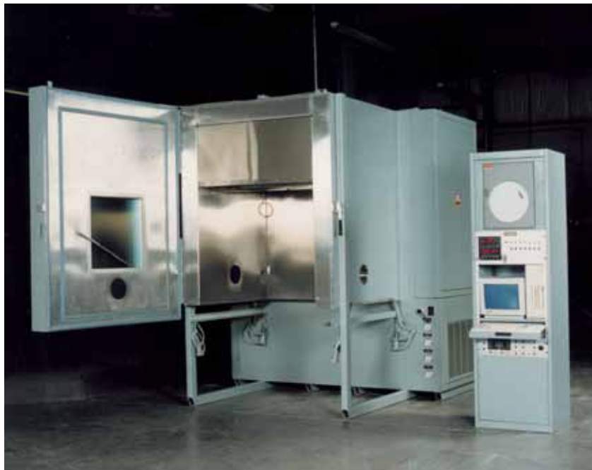
Small environmental chambers are used to research and develop process cooling application requirements. This Agree environmental chamber has a temperature range of -100 to 350°F (-73 to 177°C).
