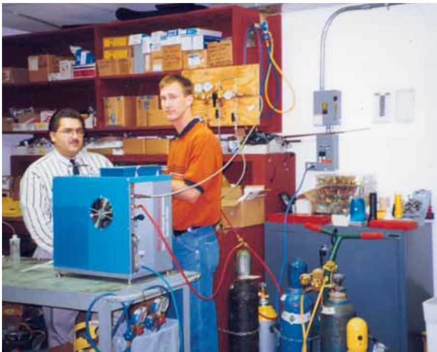
HVACR Universal certified technician Brian Burnett and Duncan Supply representative Gary Warner monitor a very-high-pressure refrigerant recovery system's cylinder evacuation process.
