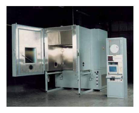
Small environmental chambers are used to research and develop process cooling application requirements. This Agree environmental chamber has a temperature range of -100 to 350°F (-73 to 177°C).
