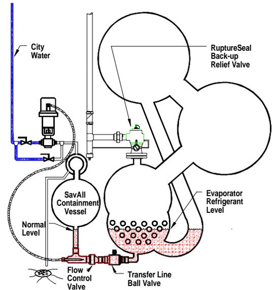
**Figure 1. - Chiller Idle, Pressure Normal**
