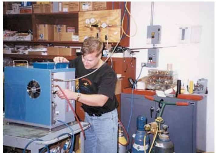
Figure 1. Certified hvac technician Erich Hibner makes the connection to a very-high-pressure refrigerant recovery unit.
